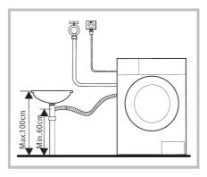
When installing the drain hose into the laundry sink, make sure it is properly fitted with rope to hold it in place. If the hose is too long, do not try to push the end were it comes from the appliance in to shorten length, this can damage it.
