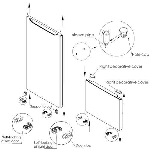
10. Install the door of refrigerator on the lower hinge and the middle hinge left side of the refrigerator and tighten the screws.Place on the shaft sleeve.Install the plug pin in the hole on the middle beam at the other end.
