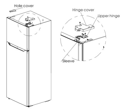
3. Unscrew the hinge screw, take of the middle hinge and the upper shaft sleeve, remove the two hinge hole covers (plug ins) on the middle hinge and take out the door body of the refrigerator chamber upswards.
