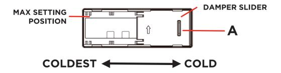
For better use of the refrigerator, it is recommended to keep the slider in original position.
