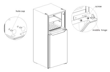
**Step 3** Remove the lower hinge assembly from lower right corner and remove the hole cap, screw cap from lower left corner; Dismantle the hinge shaft and adjustable foot and install them on the other side of lower hinge; then install the lower hinge assembly on lower left corner by fitting screws, and install the hole cap and screw cap on lower right corner.
