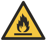
Warning: Risk of Fire/ Flammable Materials
