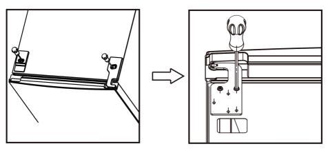
2. Unscrew from the middle hinge by screwdriver, then take off the lower door.
