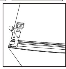
9. Take the left hinge cover from accessory bag and install it with the top hinge. Then install hole cover at right side.
