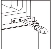
3. Tilting the refrigerator back with someone holding the back so it does not fall. Take out the does not fall. Take out the adjusting feet as shown to the right, then unscrew the lower hinge by screwdriver.
