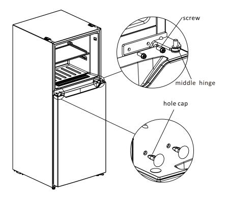
4. Remove the lower hinge assembly from lower right corner and remove the hole cap, screw cap from lower left corner; dismantle the hinge shaft and adjustable foot and install them on the other side of lower hinge. Then install the lower hinge assembly on lower left corner by fitting screws, and install the hole cap and screw cap on lower right corner.
