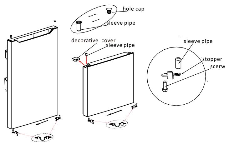
6. Install the refrigerator compartment door on the lower hinge and then install the middle hinge and hole caps.
