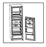
**Step 5** Remove the refrigerator door.
